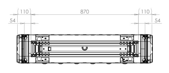
SECTION A-A SHOWING CHASSIS DETAIL
