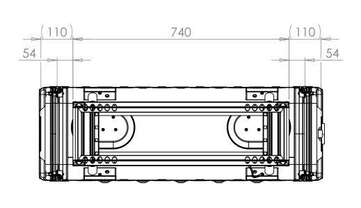
SECTION A-A SHOWING CHASSIS DETAIL
