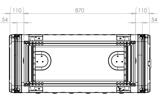
SECTION A-A SHOWING CHASSIS DETAIL
